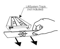
2 Examine the illustration below and proceed with the removal of the LiftSystem Track springed pin. Remove in two steps:
